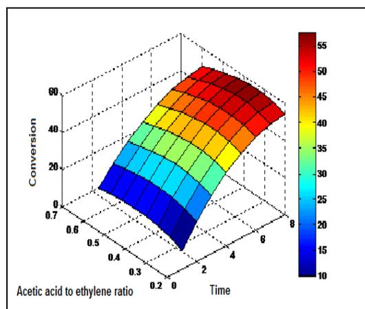
**Figure 4a:** Surface plot of epoxidation conversion as a function of hydrogen peroxide to unsaturation ethylene ratio and time at constant hydrogen peroxide and temperature of castor oil
