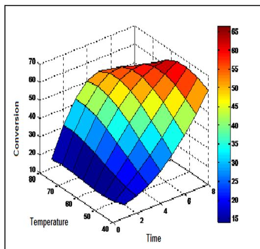
**Figure 3c:** Surface plot of epoxidation conversion as a function of temperature and time at constant both hydrogen peroxide and glacial acetic acid to unsaturation ethylene ratio of jojoba oil
