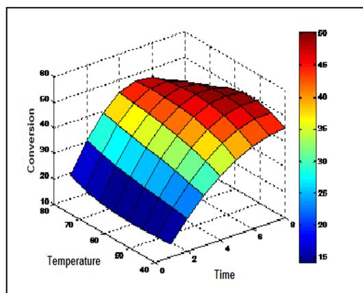
**Figure 4c:** Surface plot of epoxidation conversion as a function of temperature and time at constant hydrogen peroxide and glacial acetic acid of castor oil
