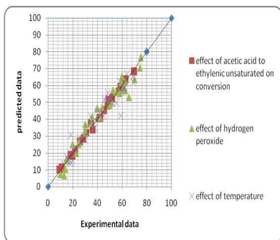
**Figure (1):** Parity plot for different introduced models for jojoba oil
