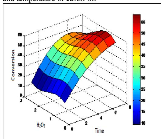
**Figure 4b:** Surface plot of epoxidation conversion as a function of hydrogen peroxide ratio and time at constant glacial acetic acid of castor oil
