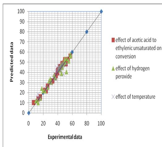
**Figure (2):** Parity plot for different introduced models for castor oil
