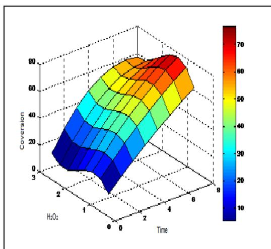
**Figure 3b:** Surface plot of epoxidation conversion as a function of hydrogen peroxide ratio and time at constant temperature and glacial acetic acid to unsaturation ethylene ratio of jojoba oil
