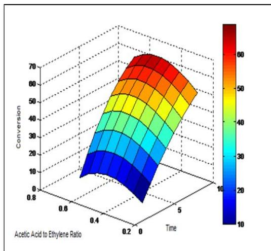
**Figure 3a:** Surface plot of epoxidation conversion as a function of glacial acetic acid to unsaturation ethylene ratio and time at constant temperature and hydrogen peroxide and temperature of jojoba oil
